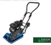
Lighter duty plate compactor 2.8 HP engine (unleaded), Plate size : 390 x 320 mm. 8,200 N compaction force. Compression depth 20 cm.
